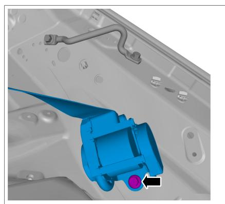
Right-hand side Remove the screw. Remove the marked part.
