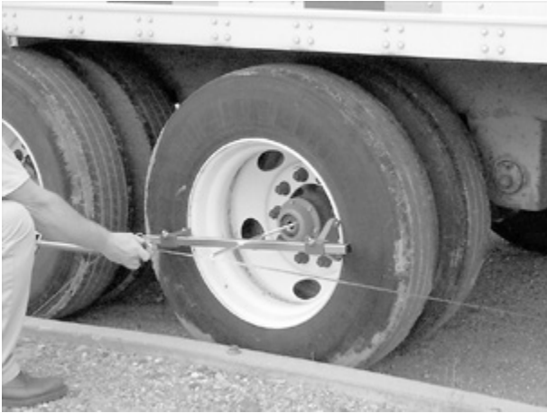
Figure 24: Measuring the "A" and "B" distances
