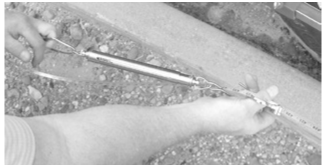
Figure 22: Using tape tension device (fish scale)
