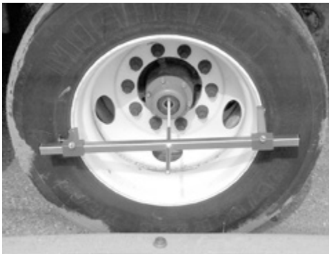
Figure 20: Installed wheel-end extender
