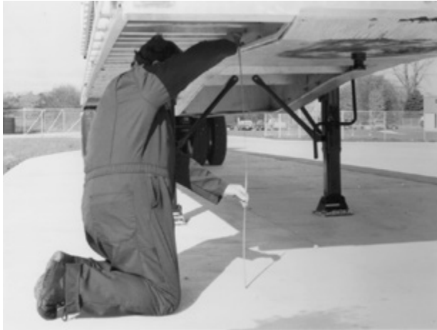
Figure 16: Measuring actual kingpin height
