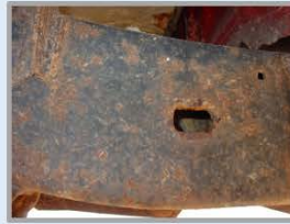
Light to Moderate Surface Rust
