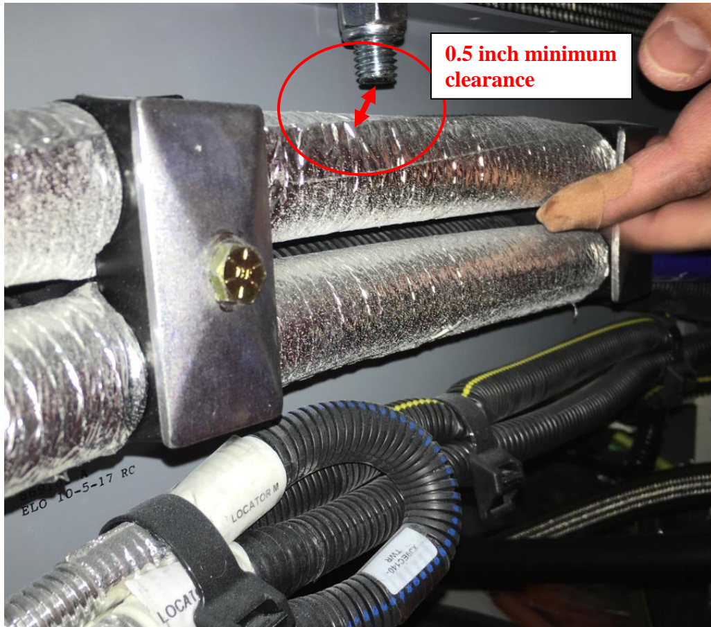
Figure 1: Gen 5 coolant lines and CAC clamp clearance goal
