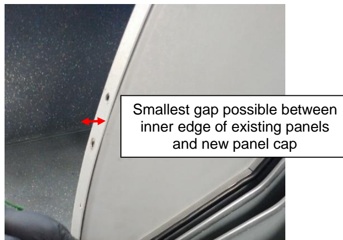
Figure 11: Achieve Smallest Gap Possible by Trimming Panel Caps if Required
