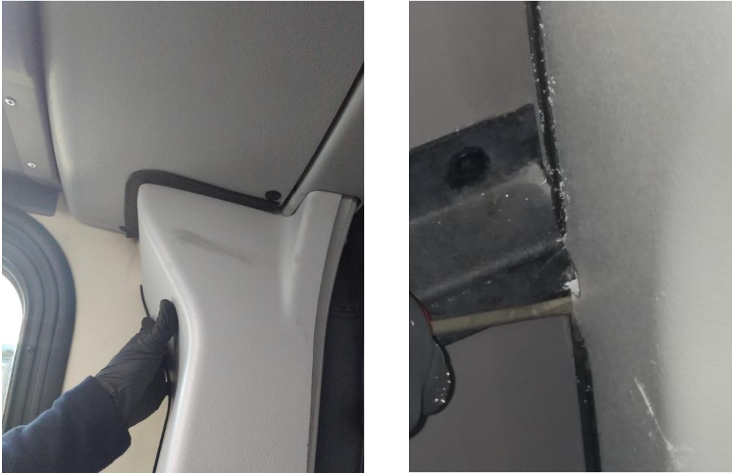
Figure 11: Dry Fit the Panels
