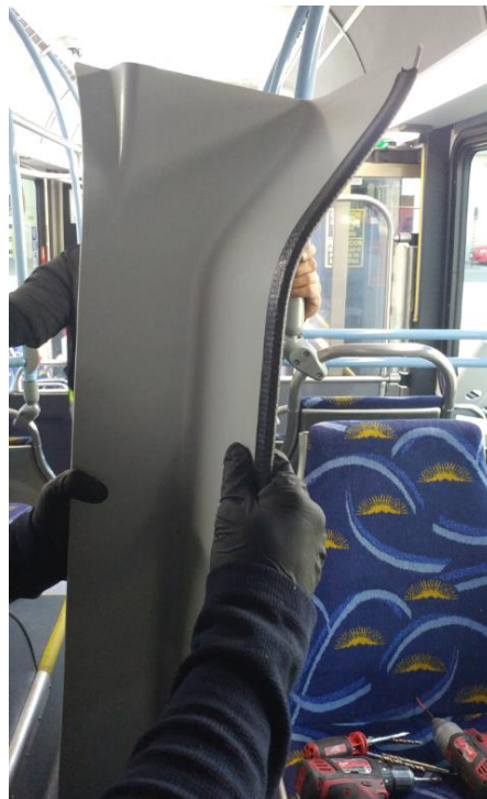
Figure 10: Install New Trim Strip
