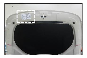
With an alcohol wipe or equivalent cleaner, clean the surface of the existing emissions label from contaminants and debris.
