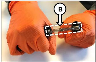
Remove and replace the RFI spring with the new improved part.
