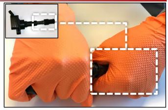
While firmly holding both ends, carefully wiggle and pull the ignition coil boot off from the igniter to expose the RFI spring (B).
