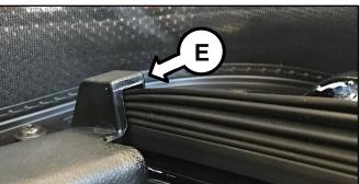
6. Ensure complete attachment of the bottom of the folding cover to the lower sliding rail.
