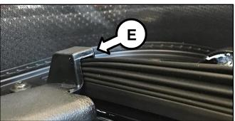
Ensure complete attachment of the bottom of the folding cover to the lower sliding rail.
