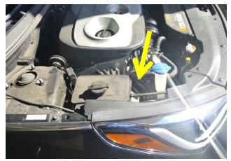
Inspect the HSG pulley nut to determine whether the paint marks line up between the nut and bolt.
