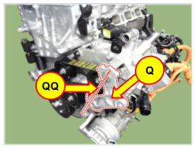
24. Install the Intake Manifold (**P**) in reverse order of removal including new gaskets, throttle body, EGR tube, PCV, and PCSV.
