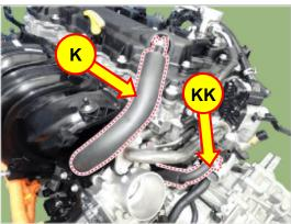
Remove the 2 bolts from the EGR cooler pipe
