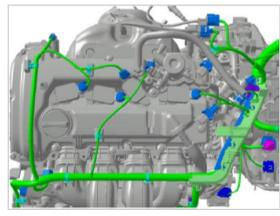
11. Disconnect the positive crankcase ventilation (PCV) hose (**K**) and the PCSV (purge control solenoid valve) hose (KK).
