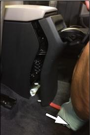
6. Move the trim removal tool to the bottom right side of the console rear cover.
