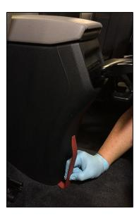
5. Rotate the trim tool down to engage the tool on the inside surface of the cover.
