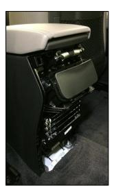
8. Remove the seven (7) screws for the cupholder assembly.
