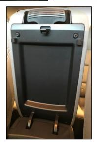
12. Reinstall the rear cover on to the floor console.
