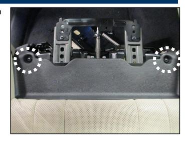
8. Remove pipe housing screws.
