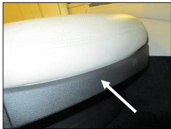
5. Remove side shield cover screw.
