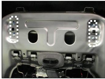
9. Lift seat cushion panel to remove tilt pipe housing.
