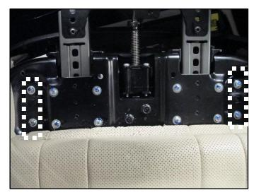
9. Lift cushion to remove tilt pipe housing.
