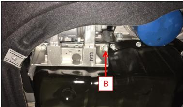
3. Verify that the A/C compressor bracket is now properly attached to the engine block and then reinstall the underbody access cover.
