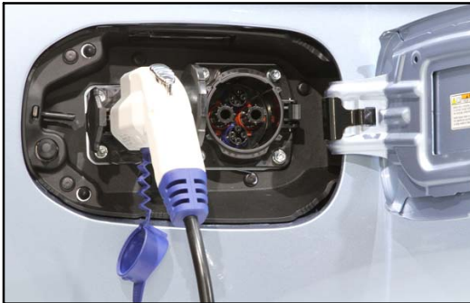
Level 2 Charging: 240V Charging Station (Eaton shown as example)
