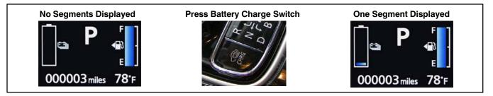
• If one or more segments are displayed, press the POWER button to enable "READY" mode and maintain for 30 minutes. This will charge the 12V auxiliary battery.
