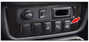
a. To enable power to the 120V AC outlets on the Outlander PHEV, press the "AC 1500W" switch in the center console.
