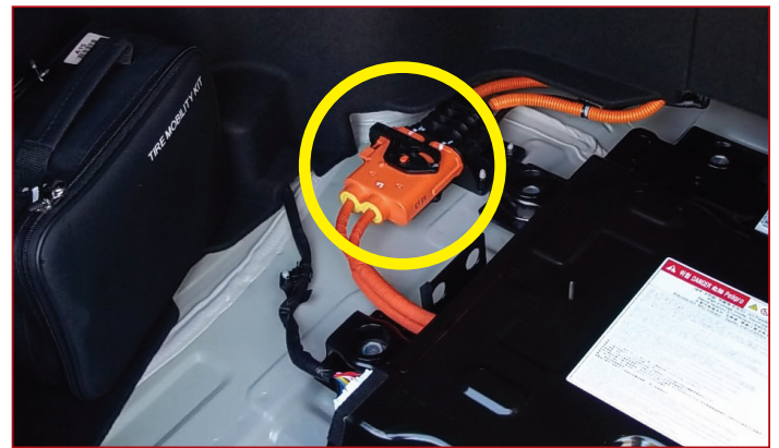
Fig. 5. Optima PHEV (JF) battery-to-battery HV connector in trunk
