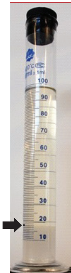
Fig. 3. This gasoline sample tested contains approximately 8% alcohol/ethanol
