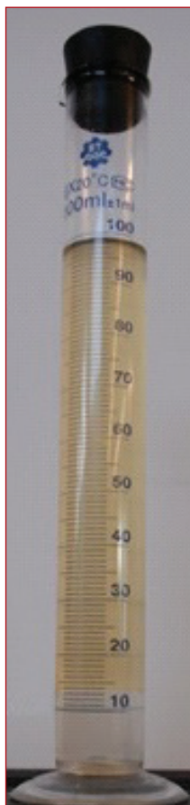
Fig. 2. Graduated glass cylinder filled with gasoline and water to the 100-ml mark showing the alcohol concentration
