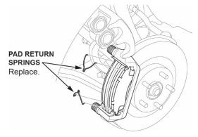
7. Remove the pad shims and the brake pads.
