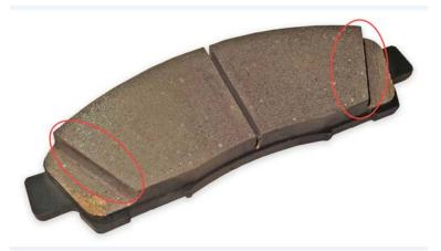
16. Apply a thin coat of M-77 Assembly paste to the **new** pad side of the shims, the back of the **new** brake pads, and the other areas indicated by the arrows shown in the picture below.
