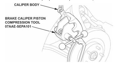
13. Press in the piston with the brake caliper piston compressor tool.
