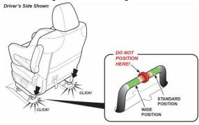
If despite the risks, a customer chooses to tip the entire second row seat forward to access the third row, they need to make sure the seat is in the standard or wide position when lowering and latching the seat.
