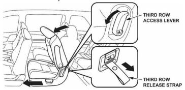
When a child seat is installed in the outer second row seats (typically using the LATCH anchors), the child seat prevents the seat-back from folding forward, which limits access to the third row. Some owners use the seat lock release lever to tip the entire seat forward with the child car seat installed to gain access to the third row.
