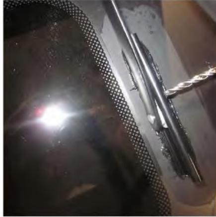
STEP 2. MOVE ROLLER AWAY FROM DRILL POINT & DRILL HOLE
