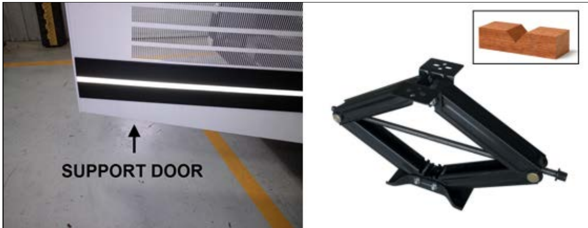
FIG.10 SUPPORTING THE DOOR
