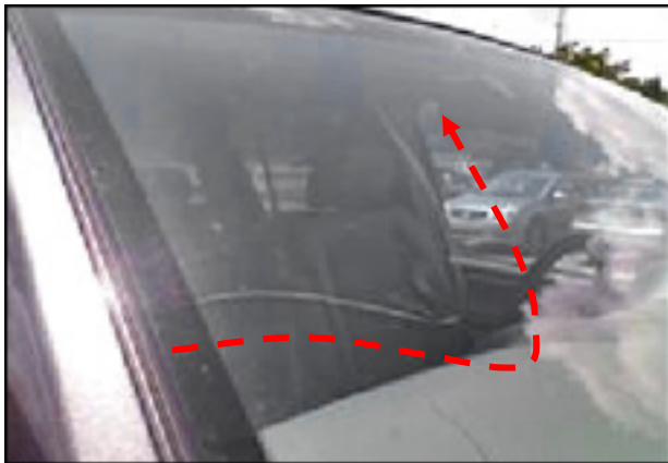
Single crack with no impact mark: Warranty
