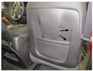
The cause of this condition may be that during cooled seat operation, a direct flow of warm air exhausts from the upper seat back ventilation heating/cooling blower thermal exchange blower unit.
