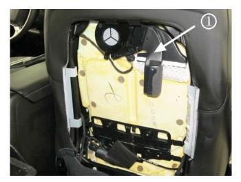
It has been found that removal of the exhaust duct (1) on the upper seat back ventilation blower allows for a less direct air exhaust and disperses t warm air more thoroughly within the seat back cushion. Remove the upper ventilation blower duct from BOTH the driver and passenger seats usin the following steps:
