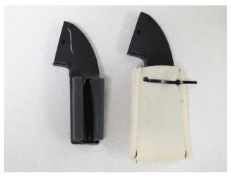
2. Locate the ventilation blower exhaust duct. Depending on the vehicle, the duct may look like either example shown in the graphic above.
