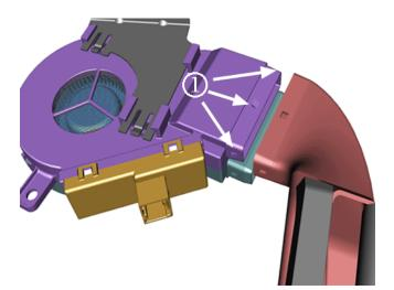
3. Grab and twist the ventilation duct to release the top and side retaining tabs (1), and remove the duct from the vehicle.
