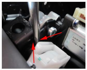
Note: You may need to move the crossbar using a flat head screwdriver to properly align the clip.
