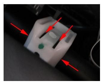
**Note:** Spray Super Lube, P/N 12346241 (in Canada, P/N 10953474), or equivalent to the areas on the white clip, as shown in the illustratic above, to ensure that the noise is eliminated.
