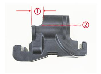
If brackets are evident, it will be necessary to remove plastic material from the top side of the guide end of the clip to enable installation. Using a grinder, or similar tool, remove approximately 10 mm (0.40 in) of material (1) from the top, down to the mold seam line (2).
