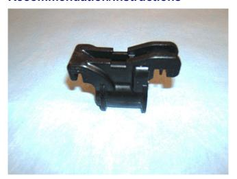
A clip has been made available to eliminate the lateral seat movement. Use the following steps to install the clip to the driver side seat. If the vehicle is equipped with a 6-way adjustable passenger seat, repeat the procedure on the passenger seat.
