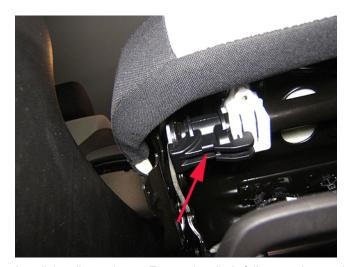
3. Install the clip as shown. Ensure the clip is fully seated around the crossbar and on the guide block.
