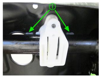
Important: On some vehicle models, a production change added welded brackets (1) to the seat crossbar on each side of the guide bloom to help retain its position. On these particular vehicles, it will be necessary to rework the new clip service part to ensure proper installation to the crossbar.
