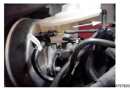
4. Disconnect the PTU vent hose assembly from the radiator surge tank assembly.
