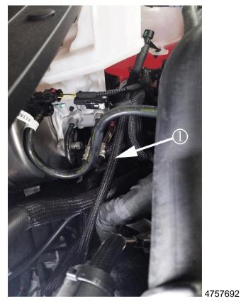
2. Locate the power transfer unit (PTU) vent hose (1).
