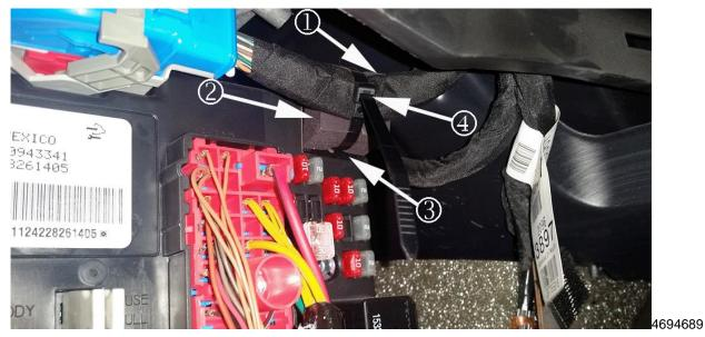
2. Apply Kent Automotive non-abrasion PET to the BCM harness, covering the tie strap just outside the X2 (C2) connector, and extending to 25 mm (1 in) past the forward corner of the BCM as shown.
