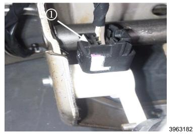
2. Disconnect the Brake Pedal Position Sensor (BPPS) connector (1).
