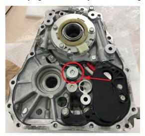
• Use a pair of needle-nosed pliers to CAREFULLY remove the relief valve from the case.
