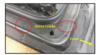
Inspect the sunroof water channels for stress cracks
