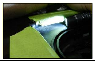
Use a flashlight at different angles to help identify any air bubbles. If any foil needs to be removed and reinstalled, discard the foil and use a new piece
