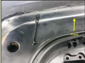
For all cracks, put a 1 mm bead of sealant (Teroson MS-930, part number D 172090A2) over any existing cracks, 1 at a time. Start the sealant bead as far under the sunroof trim as possible and pull the bead to the end of the crack.
