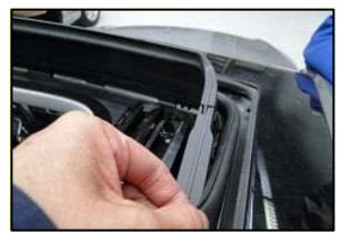
The foil must be fully applied underneath the trim panel. If the foil is folded over, it should be removed and a new piece applied. Use the squeegee to work the foil down on to the water channel as far underneath the trim panel as possible.
