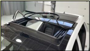
Remove the inner sunroof seal from around the front of the sunroof opening and lay it back over the sunroof glass.
