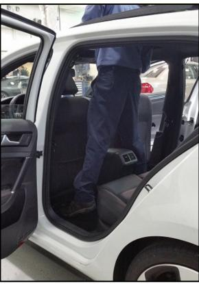
Move the front seats forward and tilt the seat backs forward to allow room to work on the roof by standing through the sunroof opening from the rear of the vehicle.
