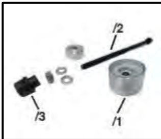
-3346- Note: 2 Spindles 3346/2 with nuts 3346/3 from assembly tool -3346-
