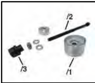
-3346- Note: 2 Spindles 3346/2 with nuts 3346/3 from assembly tool -3346-
