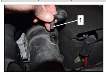
Remove low pressure hose <1> from air filter housing.
