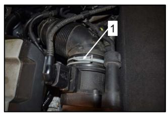
• Loosen clamp <1> to remove air duct hose.
