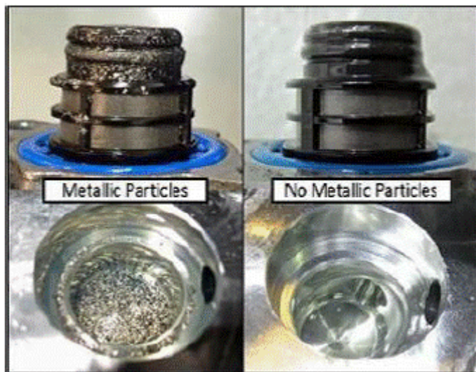
Figure 3. N290 Fuel Metering Valve and Valve Bore
