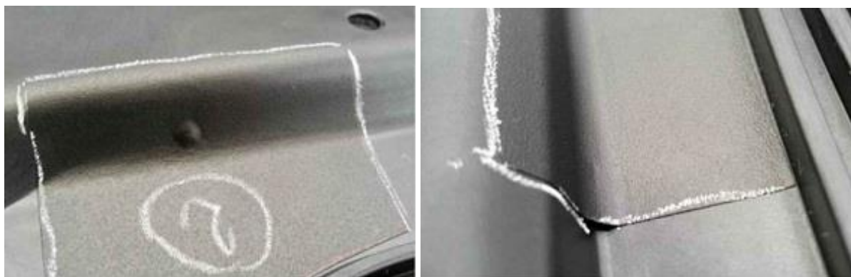
Figures 23 and 24 Air bubble under foil, air gap underneath foil.
