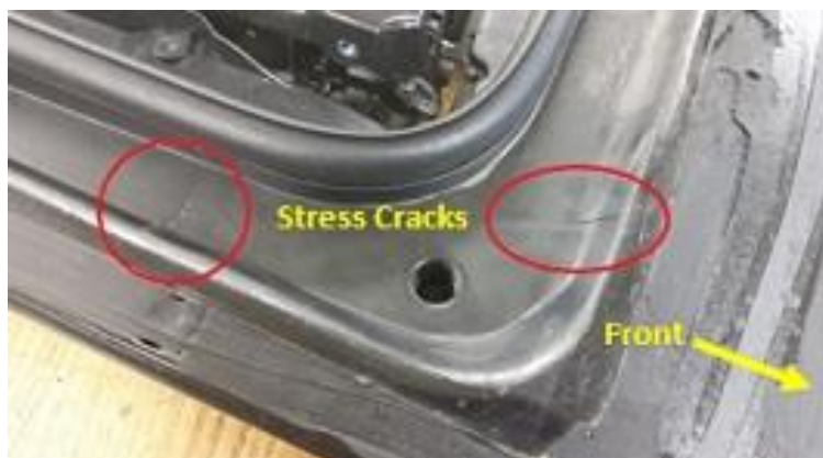
Figure 2 (Examples of stress cracks in water channel)
