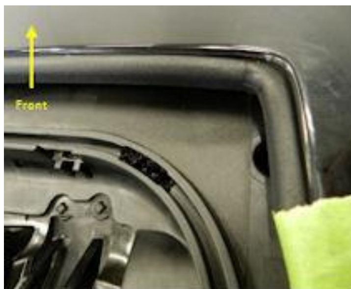
Figure 20 Foil position 5 incorrectly applied covering witness line around drain.
