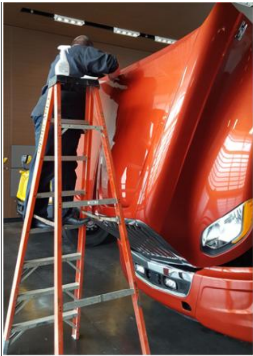
Figure #: Hood Access with Step Ladder
