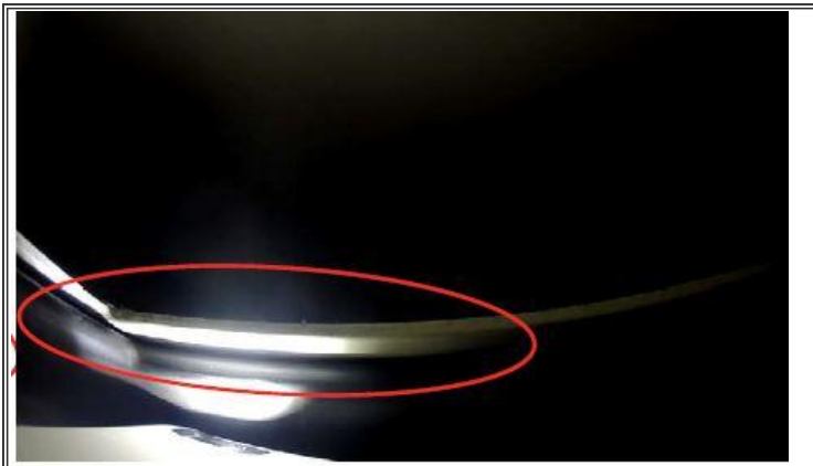
Figure 2: Hood misaligned with respect to Boot seal
