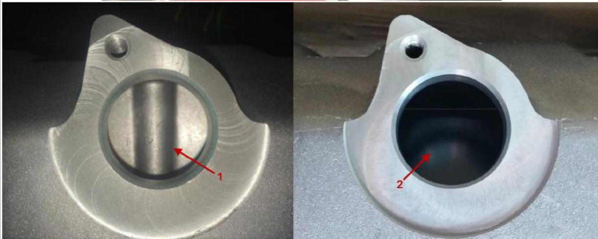
Figure 1: Valve cover baffling vs non-baffled
