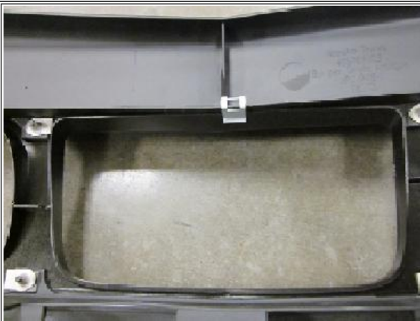
Figure 2 - Clip installation, clip centered
