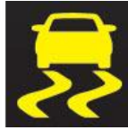
Figure 2 - Electronic Stability Control Warning Light
