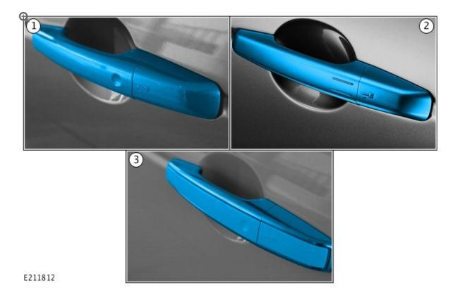
Refer to the illustration for the different handle types to make sure the correct replacement handle(s) is ordered for the vehicle.
