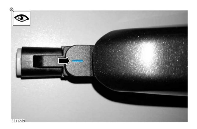
Inspect the new door exterior handle(s) for the identification mark.
