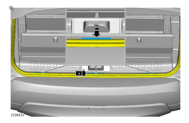
Insert the 1 shim under the tailgate seal in each position shown.
