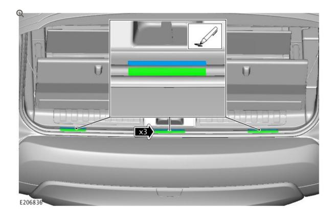
Chalk the seal where the shims are inserted.
