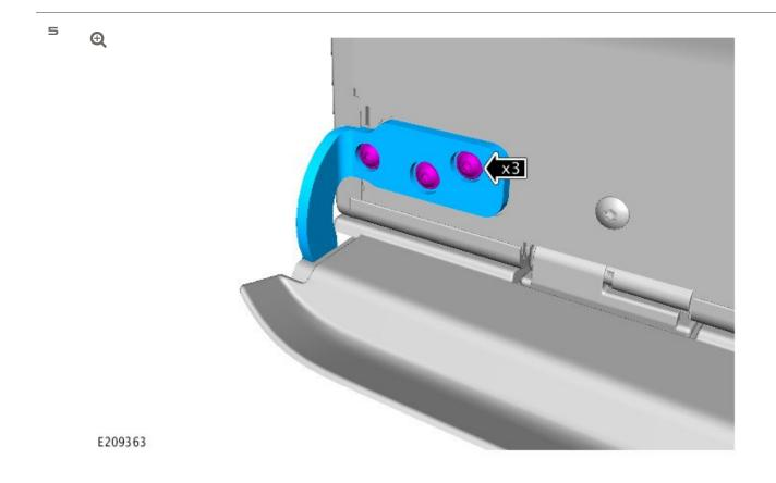
Remove and retain the 3 deployable luggage compartment floor operating arm retaining bolts.
