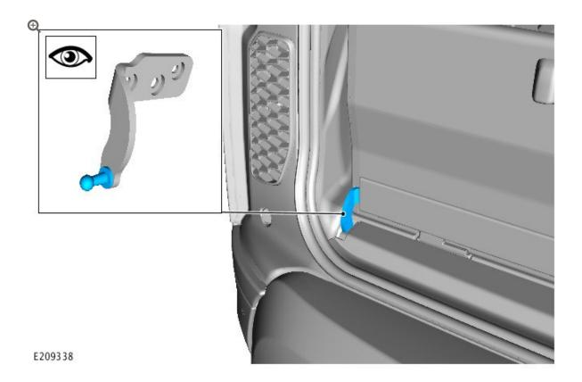
Inspect the deployable luggage compartment floor operating arm for damage (cracks/fractures).
