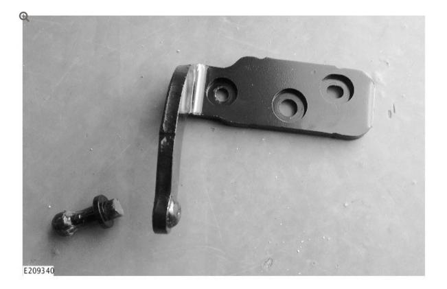
Example: deployable luggage compartment floor operating arm damage.
