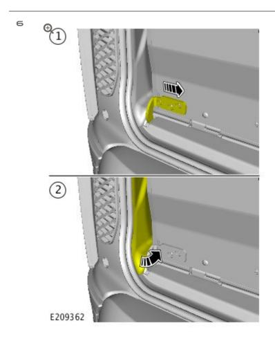
Position the deployable luggage compartment floor operating arm to the side.
