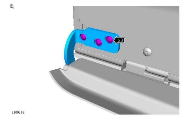
Install the 3 deployable luggage compartment floor operating arm retaining bolts.
