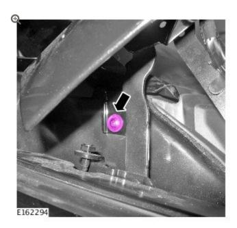
Open the hood and remove the 'A' pillar trim screw.
