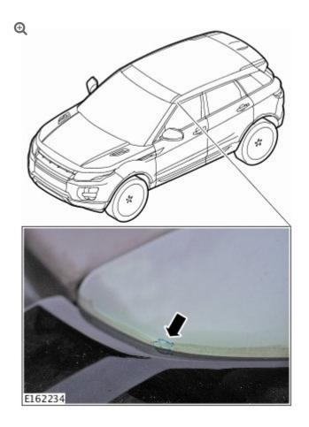
Repair and touch-up the paint in the affected area (see TOPIx Workshop Manual section 501-25: Body Repairs - Corrosion Protection).
