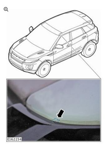
Inspect both sides of the vehicle roof panel for damage in the area shown.
