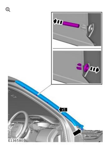
Remove the clips and then remove the 'A' pillar trim.
