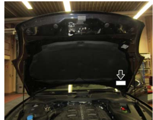
Attaching Proof of Completion label
