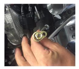
References: Workshop Manual "217119 Removing and installing oil feed line for turbocharger"
