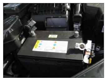
3. Remove the negative and positive battery cables.
