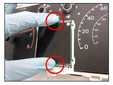
10. Press the LCD screen in until the four locking tabs are in place.
