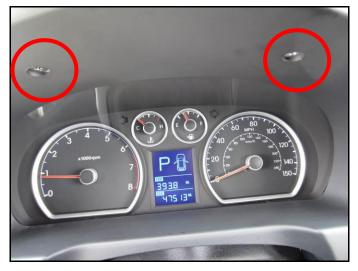
2. Remove the four screws holding the instrument cluster.
