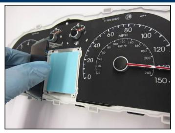
6. Lift upward and remove the blue LED light cover.
