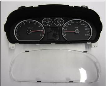
3. Carefully pinch the black locking tabs around the instrument cluster to remove the black cover.
