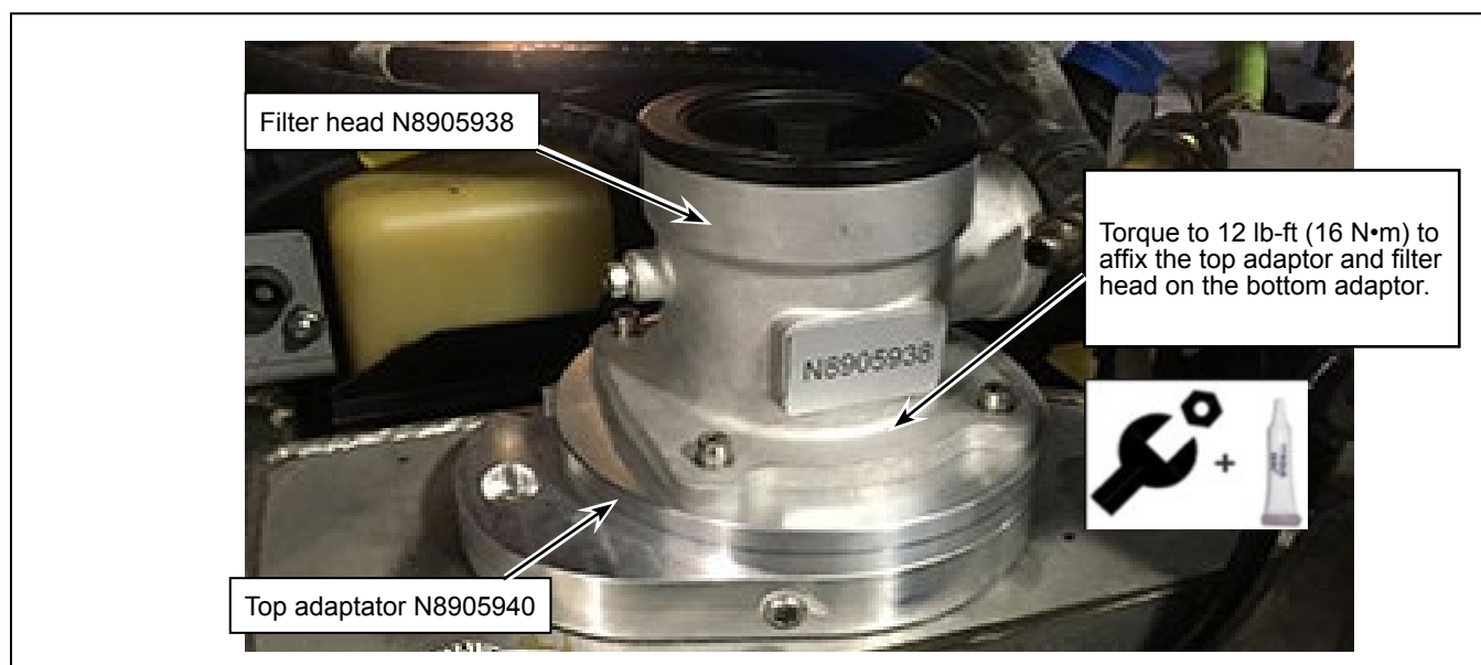
Figure 6 - Filter Head N8905938 Installed
