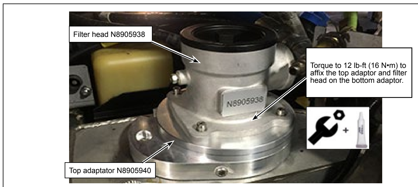
Figure 5 - Filter Head N8905938 Installed
