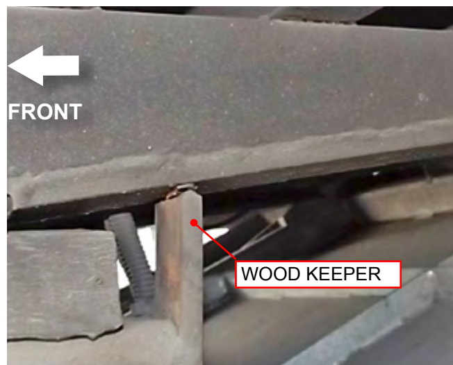
Separation at wood keeper does not affect safety of the motor vehicle. This is a non-structural component.
