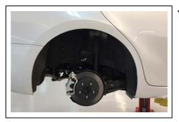
1. LIFT VEHICLE AND REMOVE RIGHT REAR WHEEL
