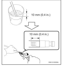
b) Immediately after removing the coupler from the hot water, twist and pull to separate the coupler from the hose using pliers and a paper towel.
