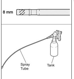
1. SPRAY GUN SET UP FOR 712AM <u>INTERNAL</u> CRC
