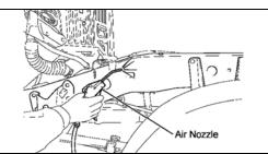
b) Use an air nozzle and remove any loose rust.
