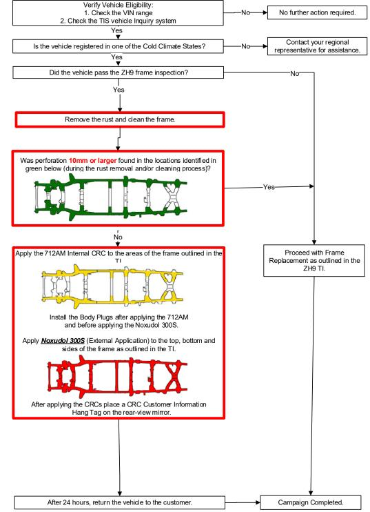
Note: Ensure to follow the entire procedure and perform all steps completely (e.g. inspection, cleaning/rust removal, CRC application, <u>one kit per vehicle</u>, etc.) any deviation will be subject to warranty claim debit.
