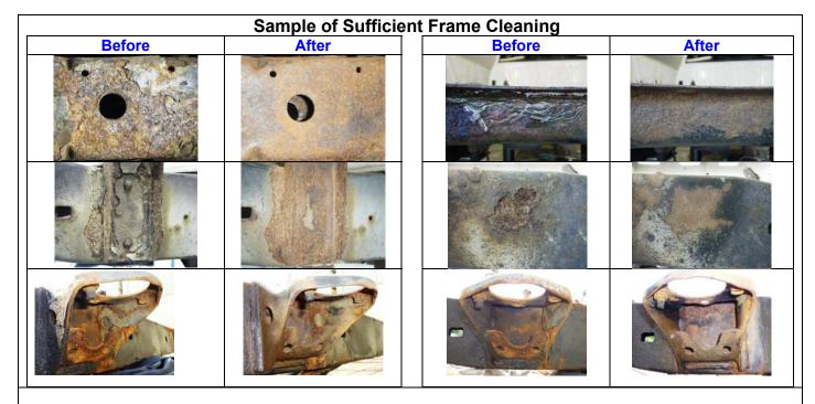
Notes : Finished surface quality of rust removal is affected with the hardness of rust. The "Hard Rust" that could not be removed by the above manner is not necessary to remove.
