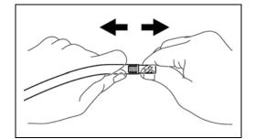
c) Holding both the nozzle and the hose pull to ensure they are securely attached.
