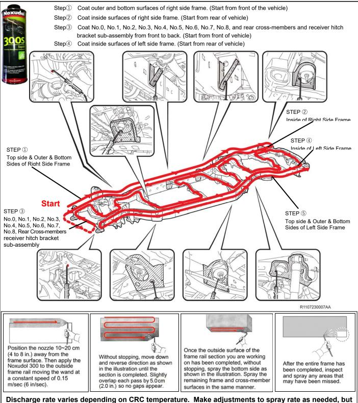
do not change air pressure (air pressure must be 50 psi).
