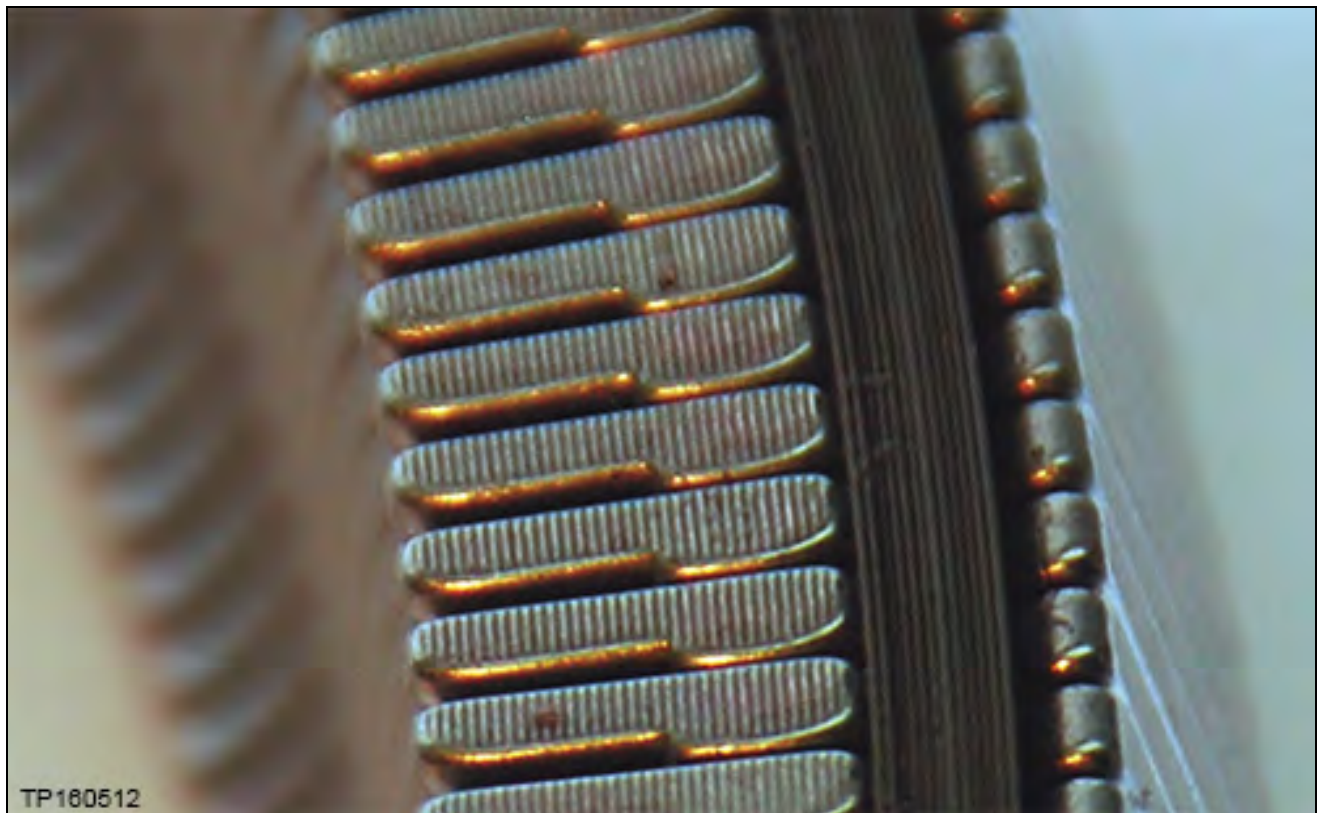
Figure 9A: Close-up of section to be inspected
