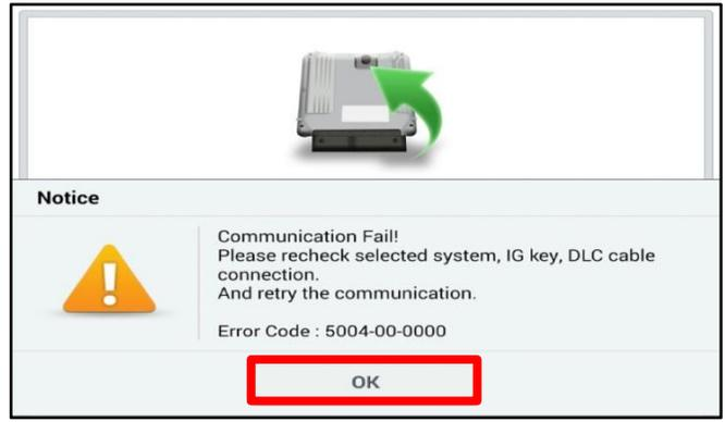
10. When instructed on the KDS, turn the ignition **OFF** for ten (10) seconds then back on. Touch **OK** to continue.
